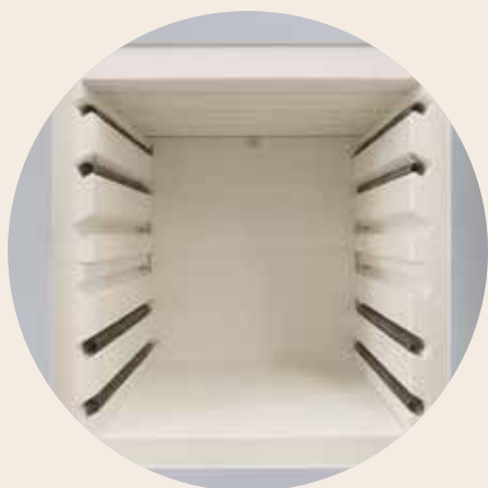
Two-sided heating with elements protected in grooves
