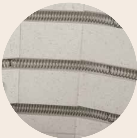
All-round heating elements, protected in grooves
