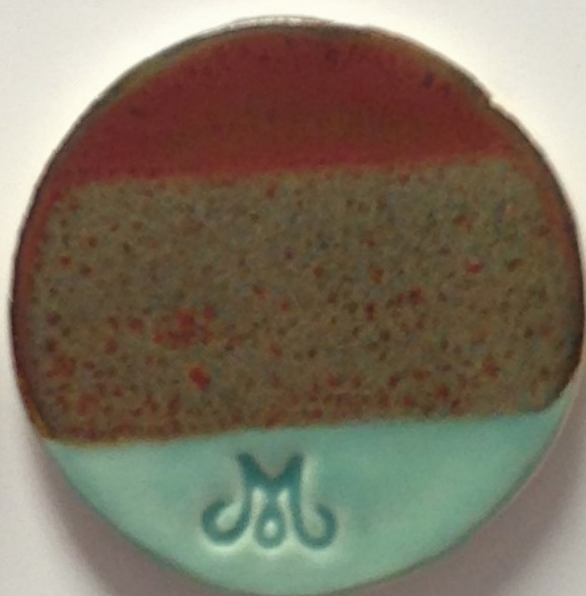
3 coats SW-130 Copper Jade Under 3 coats SW-201 Turquoise
