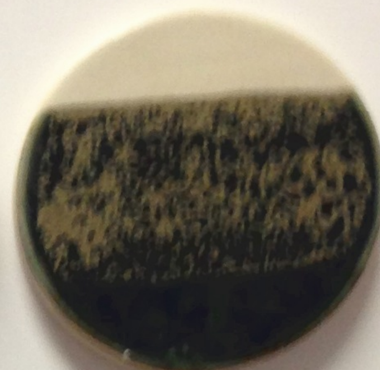
3 coats SW-120 Northern Woods Under 3 coats SW-106 Alabaster
