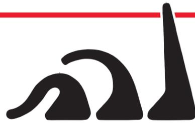
Pyrometric cones have been used to monitor ceramic firings for more than 100 years. They are useful in determining when a firing is complete, if the kiln provided enough heat, if there was a temperature difference in the kiln or if a problem occurred during the firing.
