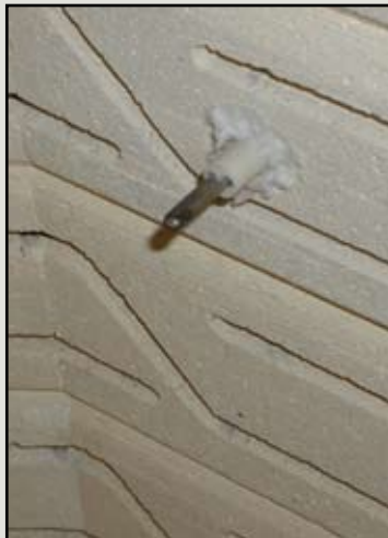
Thermocouple will show through brick wall at a maximum of 1". Pack kiln sitter hole with ceramic fiber to seal it.
