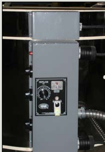
Detach screws from kiln sitter plate
